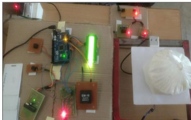
Initially it will display the quote 'select item' in the LCD. Once the product is scanned against the RFID reader, it will display the name of the product. After the product is scanned, it will display as place the product. After placing the product, it will calculate the weight of the product.
