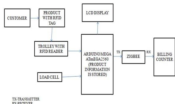
Fig 1. Architecture diagram of proposed smart trolley system
