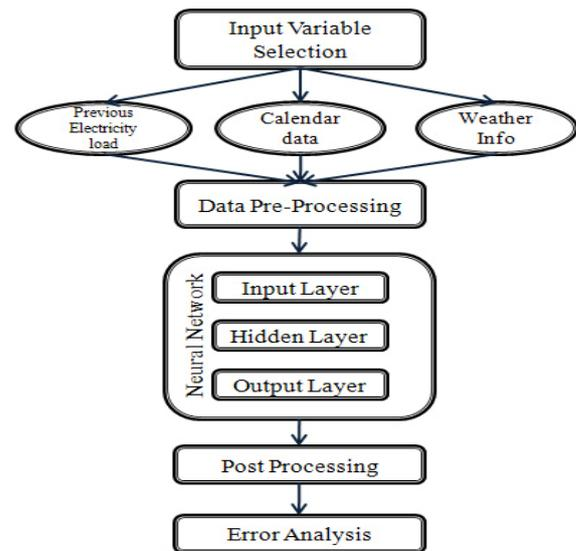
Fig. 1. Electricity load predicting system diagram
