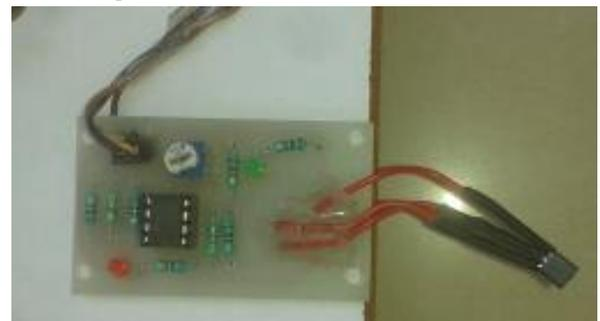
Fig 6. Temperature sensor
