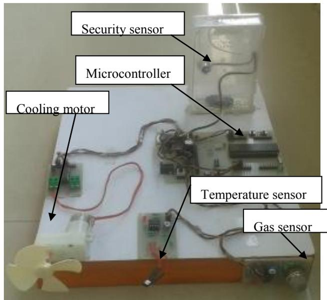
Fig 4. Test bed creation of critical sensor cluster
