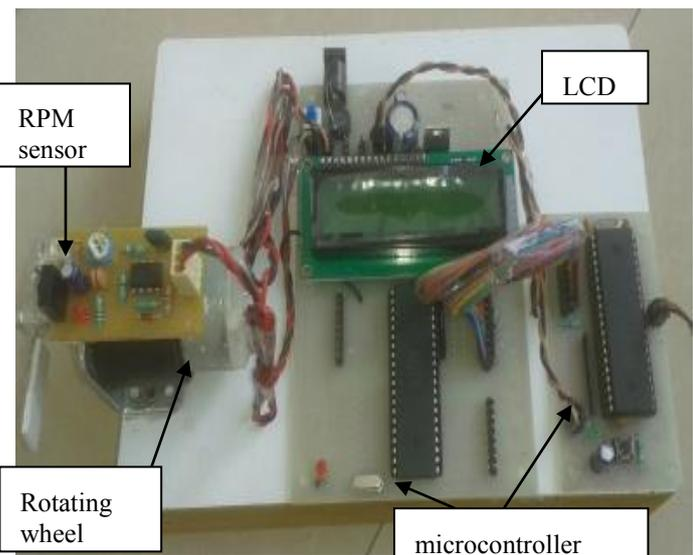
Fig 3. Test bed for creation of non critical sensor network
