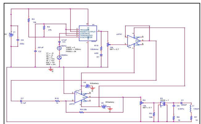
Figure 2. PSPICE model of optical interconnect model
