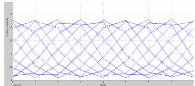
Figure 7. Eye diagram for VCSEL with sine wave input
